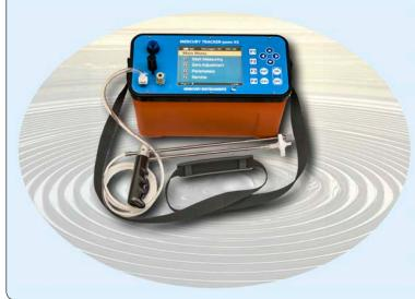
The comfortable shoulder strap allows for easy field work without fatigue. The probe makes it easy to measure the areal distribution of mercury concentrations. The probe features an ergonomic handle and is easily demountable. It can be stowed away in a separate bag.
