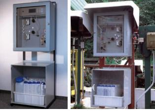
For use in harsh industrial environments: Mercury Process Analyzer PA-2
