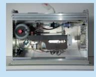
Automatic calibration unit. The system is based on mercury concentration in a saturation chamber. This concentration is automatically calculated using the mercury vapor pressure equation according to NIST.
