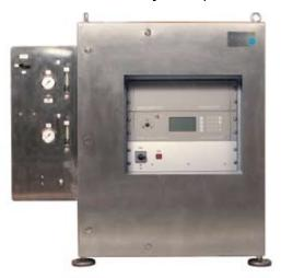
detected using atomic absorption measurement (AAS). In contrast to atomic fluorescence systems, the UT-3000 does not require special carrier gases. Air is used as a carrier gas, thus keeping the gold surface clean and enhancing the collector lifetime compared to other systems. With the UT-3000, interference from hydrocarbons or other gaseous components is insignificant (see Benzene interference diagram).
