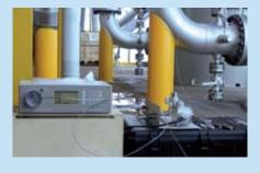
On-line field measurement of mercury in a natural gas plant. This mobile setup employs a SCS and a UT-3000 Mercury Ultratracer. The result: quick measurement of the mercury load of the gas at different points and its distribution in the process.
