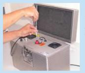
Manual calibration of the mercury analyzer. A known volume of calibration gas is drawn from the calibration device using a gastight microsyringe and injected into the analyzer's calibration port.
